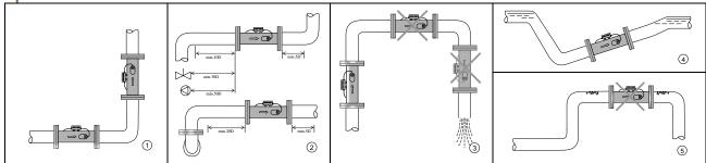
(1)Install the flowmeter on horizontal and vertical pipes
